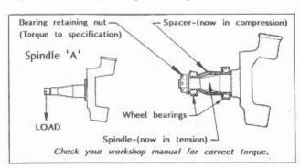
If you apply ever increasing loads to the bare stub axle spindle 'A' shown above, it will eventually bend, crack or break. . . . . . If your bearing retaining nuts are 'loose', the same thing may happen!
